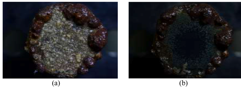
Figure 9c Specimen 12 with deposited scale: (a) before cavitation and (b) after cavitation ( \pi = 0.577(-) , \varepsilon = 0.812(-) ) (see online version for colours)
