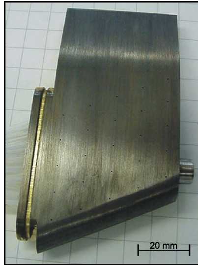
Fig. 6. ALE25 hydrofoil prepared for the measurement of static pressure.
