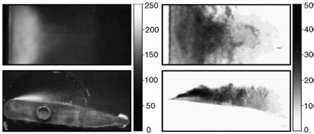
Fig. 12. Mean value and standard deviation of gray level distribution for CLE hydrofoil;  $\sigma = 2.5$ , low gas content =  $14 \text{ mg}_g/\text{l}_w$ . The standard deviation of the gray level (both side and top view) is smaller than in Fig. 11, hence we can expect less damage at the surface.
