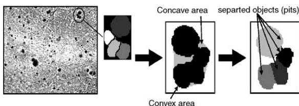
Fig. 17. Detection of pits on the surface by the pit-count method. The program recognizes the darker regions as damaged surfaces. It can also distinguish several pits that are overlapping.
