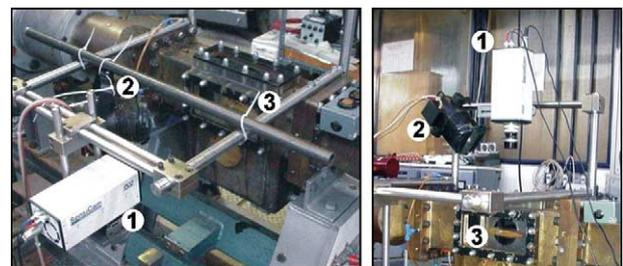
Fig. 5. The arrangement of CCD camera (1), stroboscopic light (2) and hydrofoil (3) for a side (left picture) and top view (right picture) image acquisition. It was found that the light source must be positioned at  $45^\circ$  to the camera to get the best image quality.
