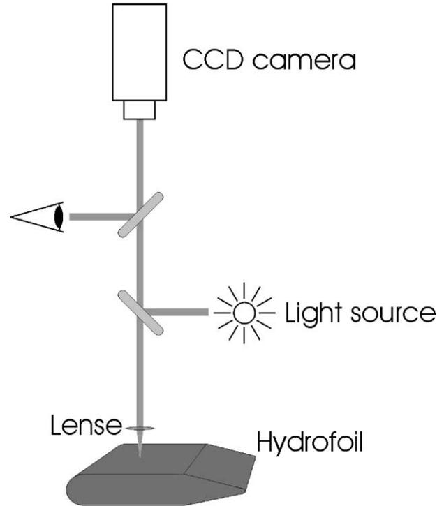
Fig. 7. Camera, microscope, light source and hydrofoil arrangement for surface image acquisition. About 925 images of the pitted surface were taken for each experiment.
