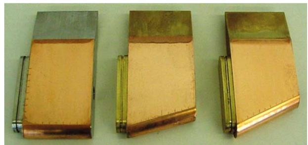
Fig. 3. Copper coated CLE, ALE15 and ALE25 hydrofoils used for the experiment. The hydrofoils are 107.9 mm long, 50 mm wide and 16 mm thick. To get some three-dimensional cavitation effects, the basic geometry was modified by sweeping back the leading edge for 15° and 25°.
