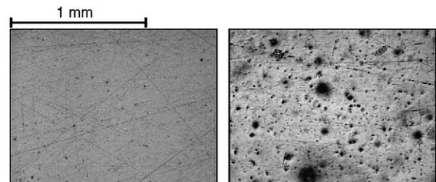
Fig. 8. Image of the surface prior (left) and after (right) the exposure to the cavitating flow. While we see no damage on the left image, almost 5% of the surface on the right image is covered with pits.
