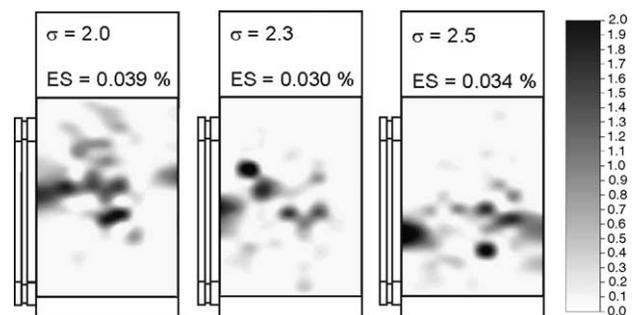
Fig. 19. Pit distribution for CLE hydrofoil, high gas content  $>45 \text{ mg}_g/\text{l}_w$ . An obvious influence of gas content can be seen. The surface sustained up to 50 times less damage when high gas content was used (comparing data in Figs. 18 and 19).
