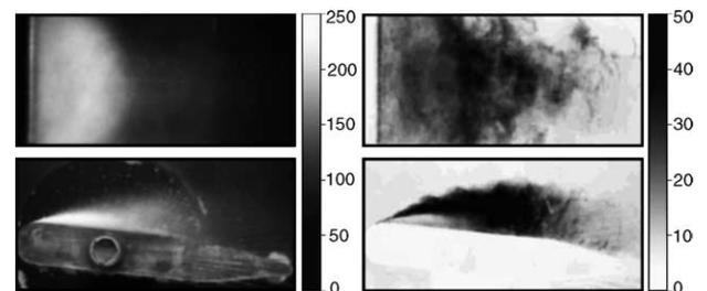
Fig. 11. Mean value and standard deviation of gray level distribution for CLE hydrofoil;  $\sigma = 2.3$ , low gas content =  $13.8 \text{ mg}_g/\text{l}_w$ . Side view distribution of standard deviation reveals that the position of the maximum is closer to the surface. It also shows a significant region with higher values of standard deviation, which suggests highly dynamical behaviour of cavitation in this region.
