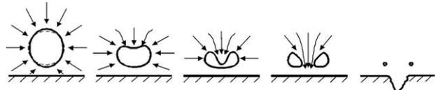
Fig. 2. Micro-jet mechanism. As a response to the pressure wave the initially spherical bubble starts to oscillate. If the oscillations are big enough the surrounding liquid penetrates the bubble and flows through it toward the solid surface. As it hits the solid surface a formation of a pit (plastic deformation) can occur.
