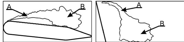
Fig. 16. Schematically presented distribution of the standard deviation distribution for the side (left) and top view (right). The source of the higher value of standard deviation in region B is cavitation cloud separation.
