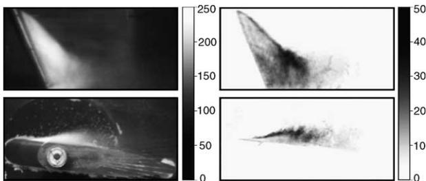
Fig. 15. Mean value and standard deviation of gray level distribution for ALE25 hydrofoil;  $\sigma = 2.3$ , low gas content =  $14.7 \text{ mg}_g/\text{l}_w$ . The distribution of standard deviation suggests that the region of where cavitation cloud separation occurs is even more specific (concentrated in the region near the front wall) than in case with ALE15 hydrofoil Fig. 14.
