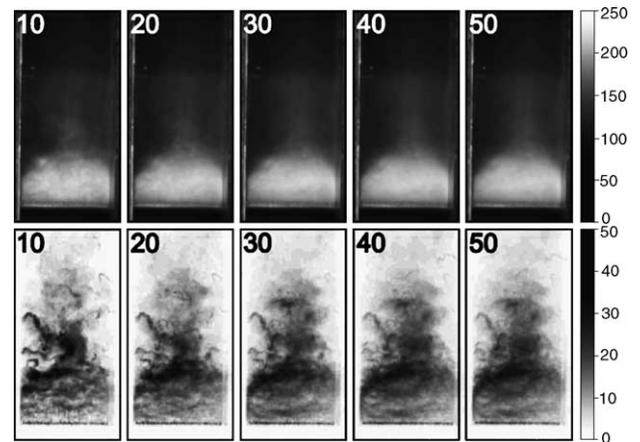
Fig. 9. Convergence test for mean value (upper images) and standard deviation (lower images) of grey level (top view). It can be seen that almost no change in the mean value of gray level or in the standard deviation of gray level can be seen after considering more than 30 images.
