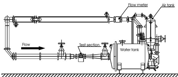
Fig. 4. Cavitation tunnel. The test section is 500 mm long 100 mm high and 50 mm wide. The maximal flow velocity is 20 m/s. The pressure at the inlet to the test section can be adjusted between 0.2 and 5 bar.
