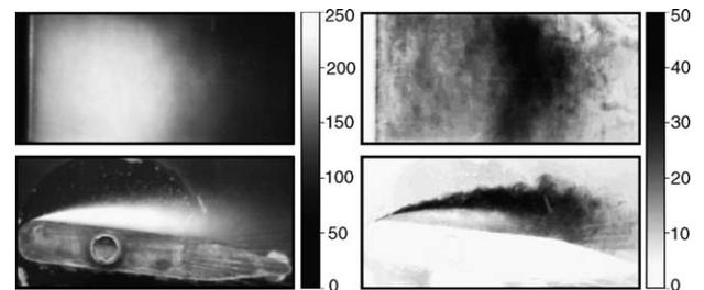
Fig. 10. Mean value and standard deviation of gray level distribution for CLE hydrofoil;  $\sigma = 2.0$ , low gas content =  $14 \text{ mg}_g/\text{l}_w$ . Observing the side view we can see that the maximum of standard deviation is far away from the surface of the hydrofoil. The larger distance contributes to lower damage of the surface (observing Fig. 18).
