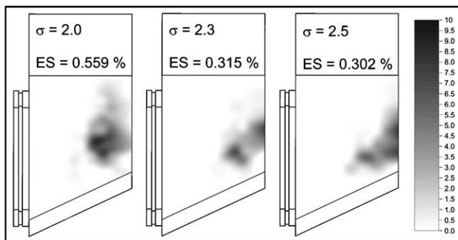
Fig. 21. Pit distribution for ALE25 hydrofoil, low gas content  $< 15 \text{ mg}_g/\text{l}_w$ . The relation between cavitation cloud shedding and cavitation damage is even more obvious in the case of ALE25 hydrofoil (in comparison to the ALE15 hydrofoil; Fig. 20).
