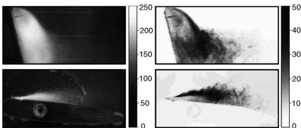
Fig. 14. Mean value and standard deviation of gray level distribution for ALE15 hydrofoil;  $\sigma = 2.3$ , low gas content =  $14.5 \text{ mg}_g/\text{l}_w$ . Looking the top view distributions we can see that the maximum of standard deviation is in the region close to the front wall (where the hydrofoil is the shortest), which relates very well to the region where we have dynamical cavitation (cloud separation, observing Fig. 6).
