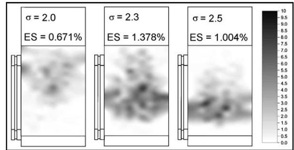
Fig. 18. Pit distribution for CLE hydrofoil, low gas content  $<15 \text{ mg}_g/\text{l}_w$ . The maximum of damage moves away from the leading edge as cavitation number is decreasing. The position of the maximum of damage corresponds to position of cavitation cloud separation, characterised by higher value of standard deviation (Figs. 10–12).
