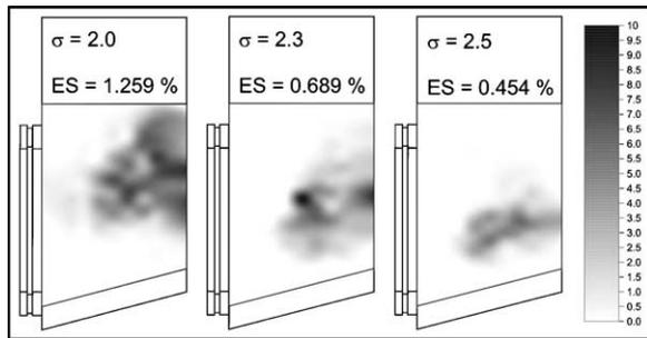
Fig. 20. Pit distribution for ALE15 hydrofoil, low gas content  $< 15 \text{ mg}_g/\text{l}_w$ . Results show that the cloud separation is a needed condition for cavitation damage. The hydrofoils were significantly damaged only in the region where cavitation cloud separation occurs.
