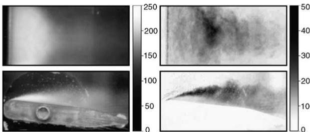
Fig. 13. Mean value and standard deviation of gray level distribution for CLE hydrofoil;  $\sigma = 2.3$ , high gas content =  $48.9 \text{ mg}_g/\text{l}_w$ . We can see that the cavitation grows when the gas content is increased. Also, the lower values of standard deviation suggest less dynamical behaviour.
