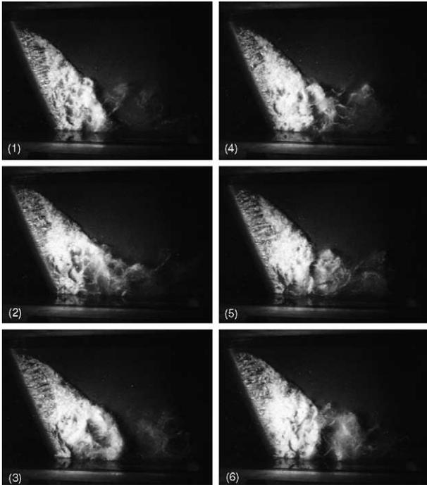
Fig. 6. Sequence of top view images for ALE25 hydrofoil. The flow is from left to the right. Significant dynamic cavitation behaviour can be seen near the front wall, while the cavitation at the rear wall remains nearly steady.
