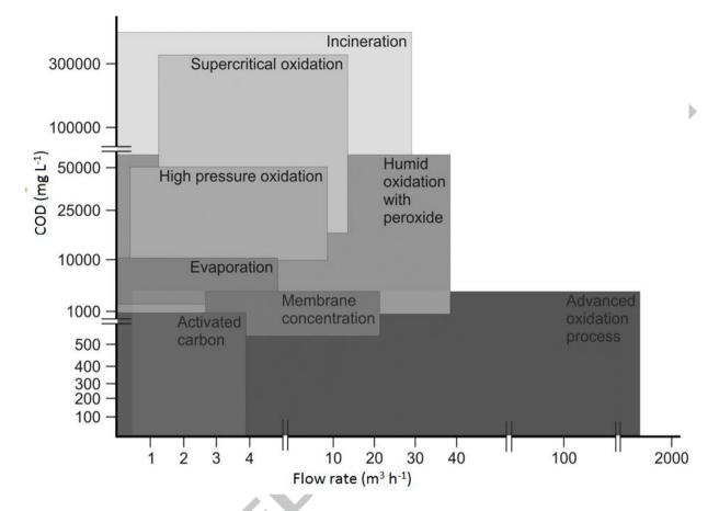
Suppl. 1: Typical technology selection chart (COD versus effluent flow rate, adapted from [41]).
