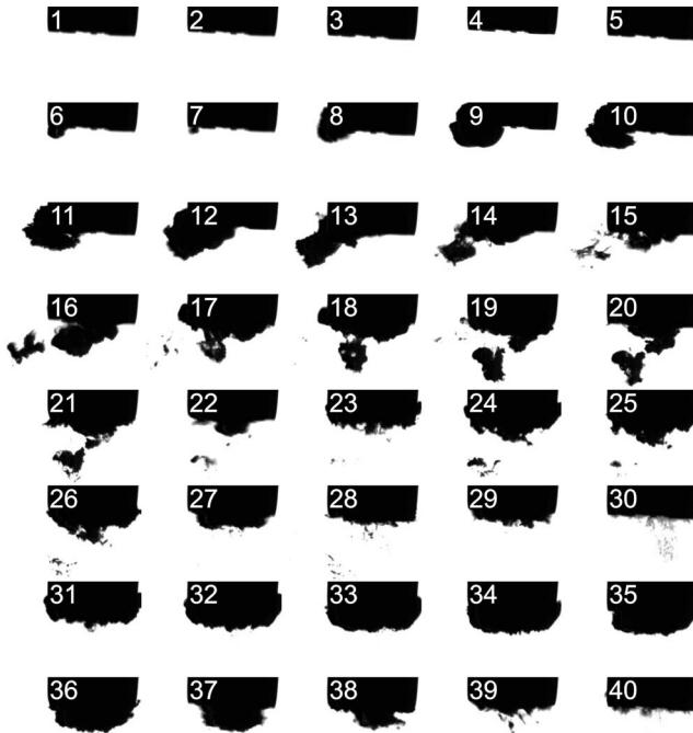
FIG. 9. Images of cavitation cloud for the lowest saturation level (20%) at startup (images with inter-frame interval of  $20 \mu\text{s}$ ).
