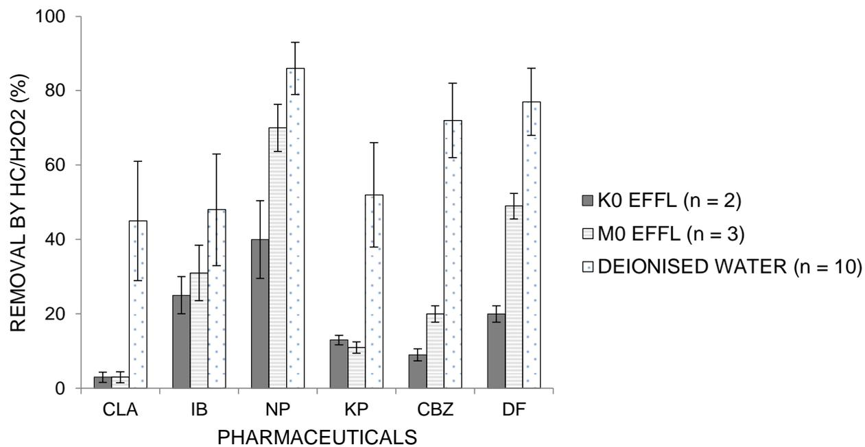
**Fig. 3.** Removal of pharmaceuticals with HC/H<sub>2</sub>O<sub>2</sub> process in K0 and M0 effluents and deionised water expressed as average removal  $\pm$  stdev (n = number of measurements).
