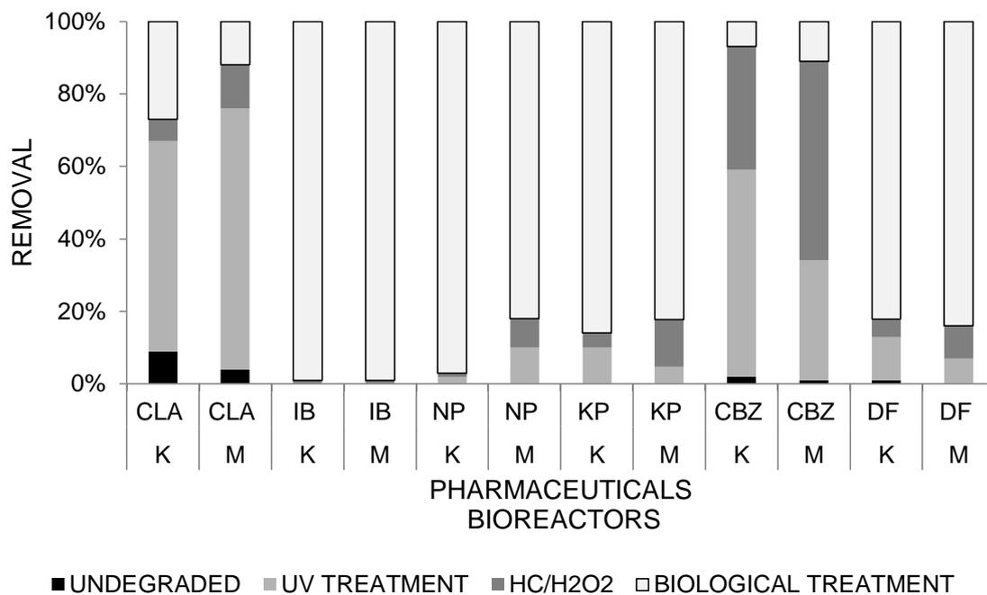
**Fig. 4.** Contributions of biological, HC/H<sub>2</sub>O<sub>2</sub> and UV treatment on overall removal of pharmaceuticals (K = K1, K2 effluent; M = M1, M2 effluent).
