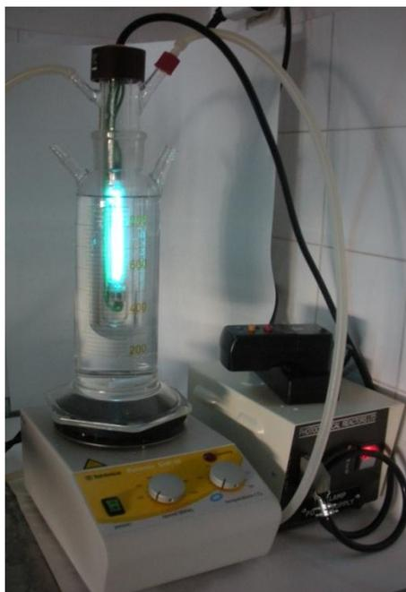
**Suppl. 4:** Cylindrical glass reactor used for UV treatment experiment.
