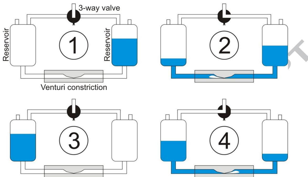
Fig. 1. Cyclic operation of the HC reactor.
