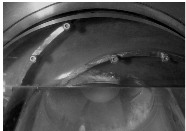
Fig. 6 View into the impeller at the investigated operating point ( q = 1.17 , \text{NPSH} = 4 \text{ m} )
